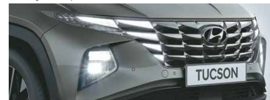
Dark chrome parametric front grille with parametric hidden LED DRLs, LED MFR headlamps & positioning lamps
